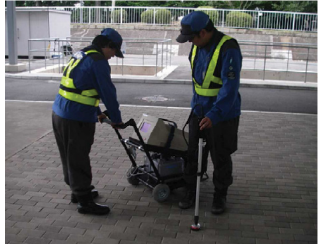
Inspectors using the transmission-type leakage detector
