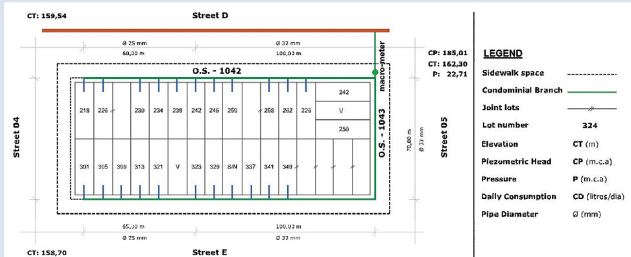
Design of condominial water distribution network in a residential block in Parauapebas
